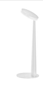
Table lighting fixture for interiors, with swivelling light beam. Pickled sheet metal bearing base in polyacrylic paint. Body in tapered steel tube in white, black, bronze, mat brass or titanium polyacrylic paint. Turned brass joint in polyacrylic paint. Die-cast aluminium structure in polyacrylic paint. Die-cast aluminium swivelling head in polyacrylic paint. Modelled acrylic diffuser with mat finish.
